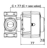
Installation dimensions for Actuator Series ARA600 with ESBE VRG100, VRG200, VRG300 and VRB100 mixing valves
