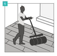
Not later than 30 minutes after gluing the panels, use a heavy roller in order to press the glued panels to the substrate ccurately and evenly.
